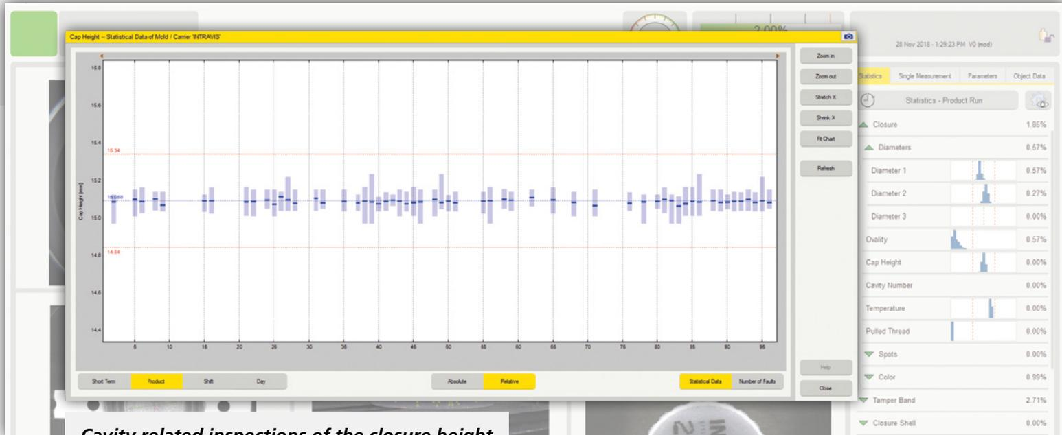
*Cavity related inspections of the closure height and spread within the tolerance borders*
