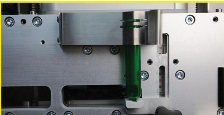
Preform jig: The object has to be inserted into the slot to determine and adjust the body length setting
