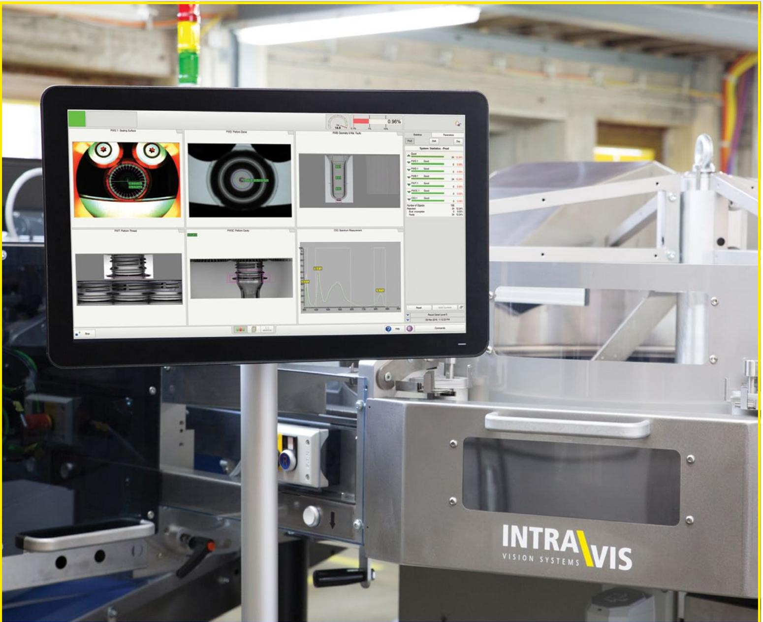
The new 16:9 HMI allows more inspection modules to be displayed side-by-side
