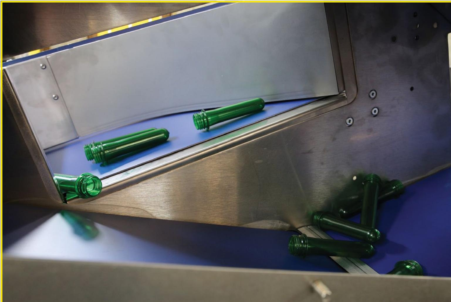
The two way conveyor provides a safe transportation, optimizing preform closing into the centrifugal feeder
