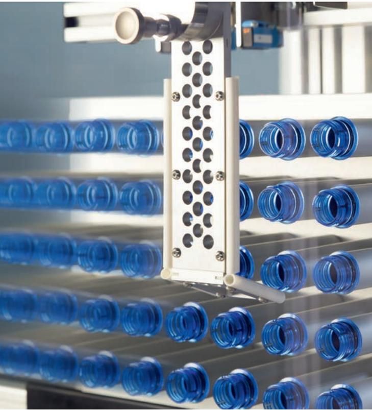
**FIG 1:** The ColorWatcher Integrated by Intravis is implemented directly into the production machine, inspecting preforms right after they are produced.
