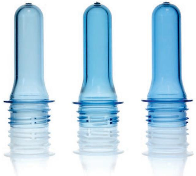
**FIG 2:** Color deviations belong to the most frequent defects in preform production. Only the middle preform has the right color - the left one is too light, the right one too dark.
