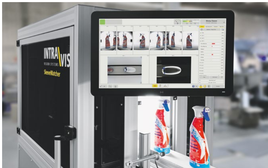
Vision system for the detection of sleeve-specific defects
