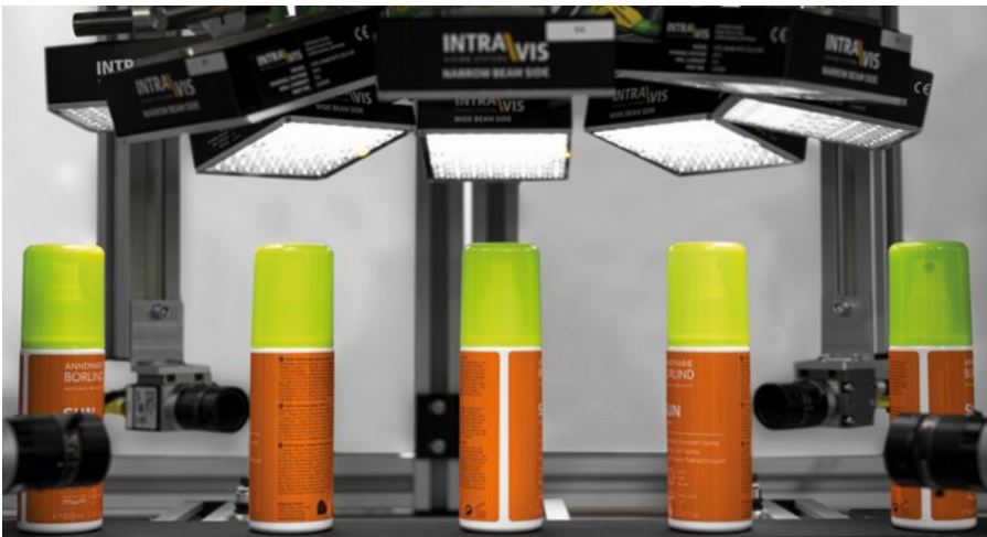
Label inspection for unoriented objects - LabelWatcher 360°
